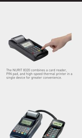
Peripherals such as the NURIT 222 PIN pad or a check reader attach quickly and
