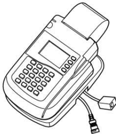
The telephone line pigtail lets you conveniently configure a direct telephone line connection without removing the swivel stand. To set up a direct connection using the pigtail cable:
