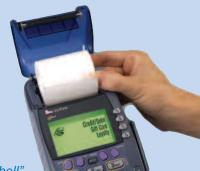
A "clam shell" printer facilitates drop-in paper loading, virtually eliminating paper jams.
